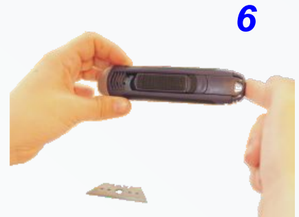
6 'Click' the end cap into place - the knife is ready to use !
