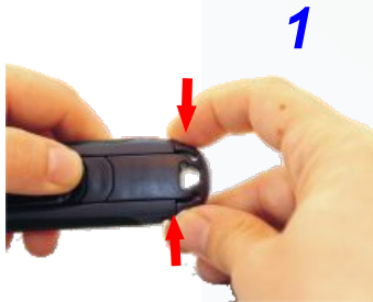
1 Press the two tabs on the rear end cap to release the cap
