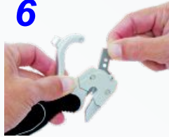
6 Slide the two new blades into their guide
