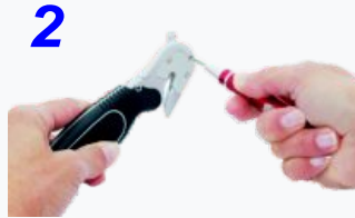
2 Unscrew the screw on the side of the aluminium head
