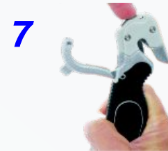
7 The blades are in place when they touch the bottom of the guide
