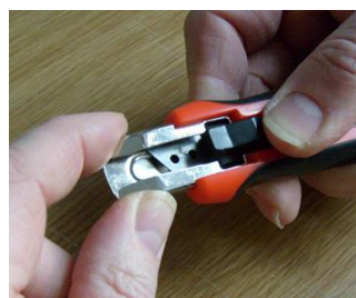
5. Align slider with cut outs and hole in blade ensuring location
