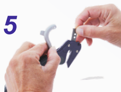
5 Remove the two used blades
