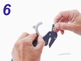
6 Slide the two new blades into their guide
