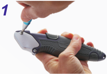
1 Remove the screw at the top of the handle
