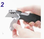
Open the head and remove the used blade
