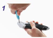
Remove the screw at the top of the handle
