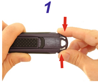
1 Press the two tabs on the rear end cap to release the cap
