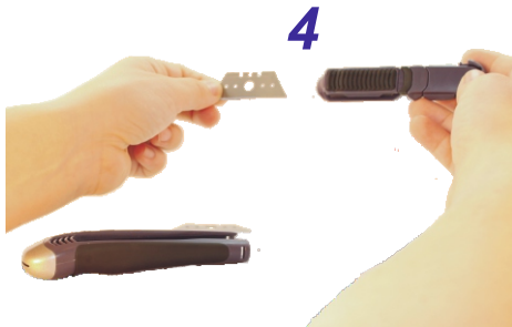
4 Locate the new blade by placing on the magnets with centre hole engaged (invert blade to change from right to left hand)
