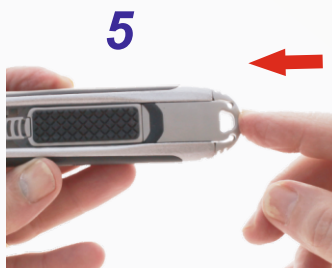
5 Replace the mono block slider
