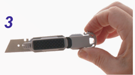
3 remove the used blade and discard safely
