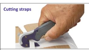
For cutting packaging tape pierce the tape with the serrated blade and pull the knife towards you.
