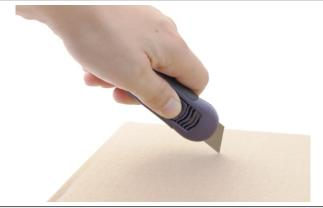
During the cut ensure the slider is released (the blade is kept deployed by friction of the material being cut).
